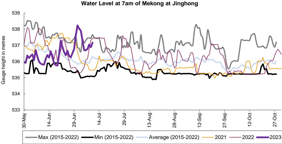
**Figure 7.** Water level at the Jinghong hydrological station up to 10 July 2023.
